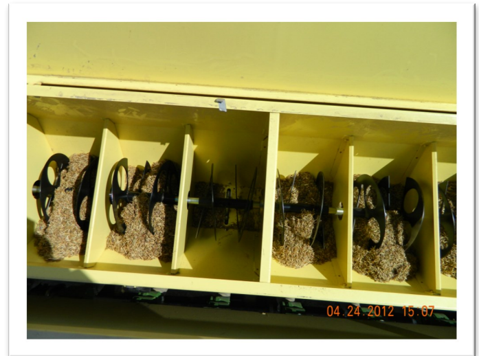
Fig. 2. Seed box with an agitator. Photo by J. Soper
